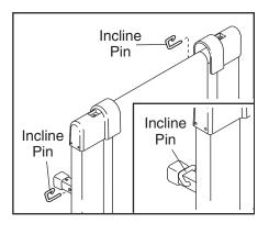
sure that the incline pin is in the "locked" position shown in the inset drawing. Adjust the other incline leg in the same way. CAUTION: Before using the treadmill, make sure that both incline legs are at the same height and that both incline pins are fully inserted from the direction shown. Do not use the treadmill with the incline pins removed.
